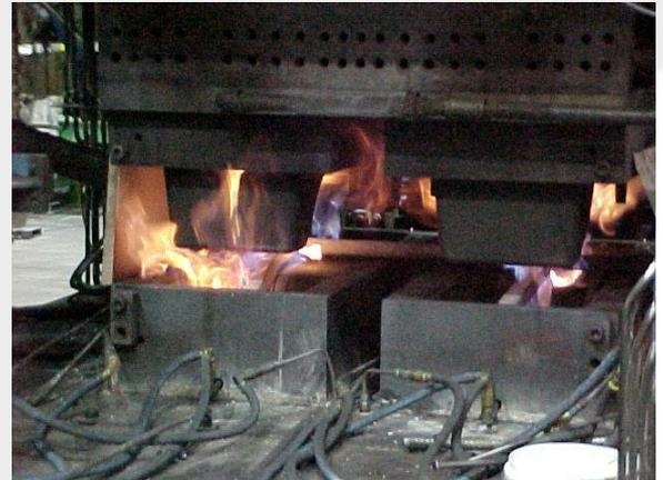
Picture no. 1: Cup burners or open flames preheating the casting die, leading to unequal preheating of the two parts of the die and creating hot spots.
