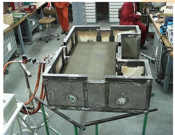
Picture no. 2: The Metal Fibre Burner with two firing sides, atmospherically fired.
