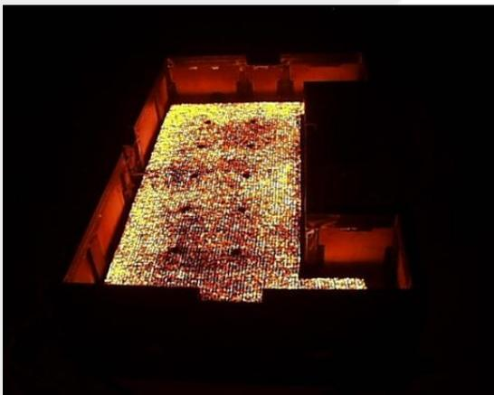
Picture no. 4: A double faced Metal Fibre Burner for the preheating of a casting die with a particular shape. The burner is over 1000 mm wide with a power output of 80 up to 250 kW with gas pressures up to 400 mbar. The burner is mounted in a box to automate insertion within the casting die.
