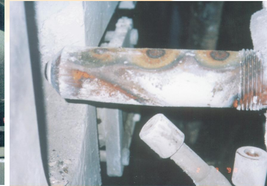
Pouring throats heated with cup burners
