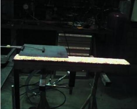
Picture no. 3: Tests with burners for determination of power output and radiant efficiency.
